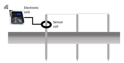
Earthpit sensor unit comprises of two major parts, viz. sensor magnetic coil and electronics processing unit. Both parts are connected through a cable, conduit, and gland arrangement. Electronics processing unit is enclosed with an IP67 plastic enclosure and named as Vadict IoT Sensor unit.
